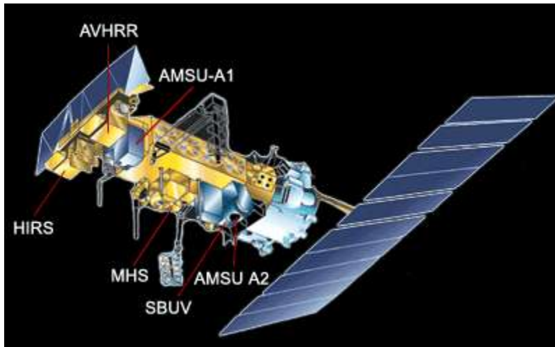
NOAA satellite and its payload
