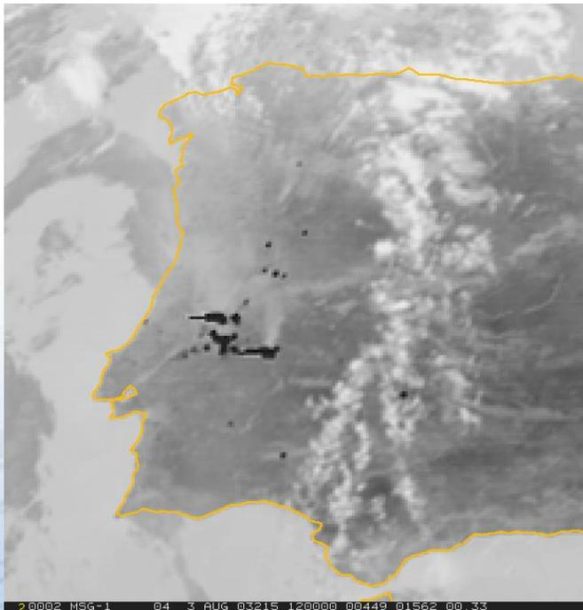
For pixels west of the fire the sensors can be blinded, following geometrical patterns (rings)
