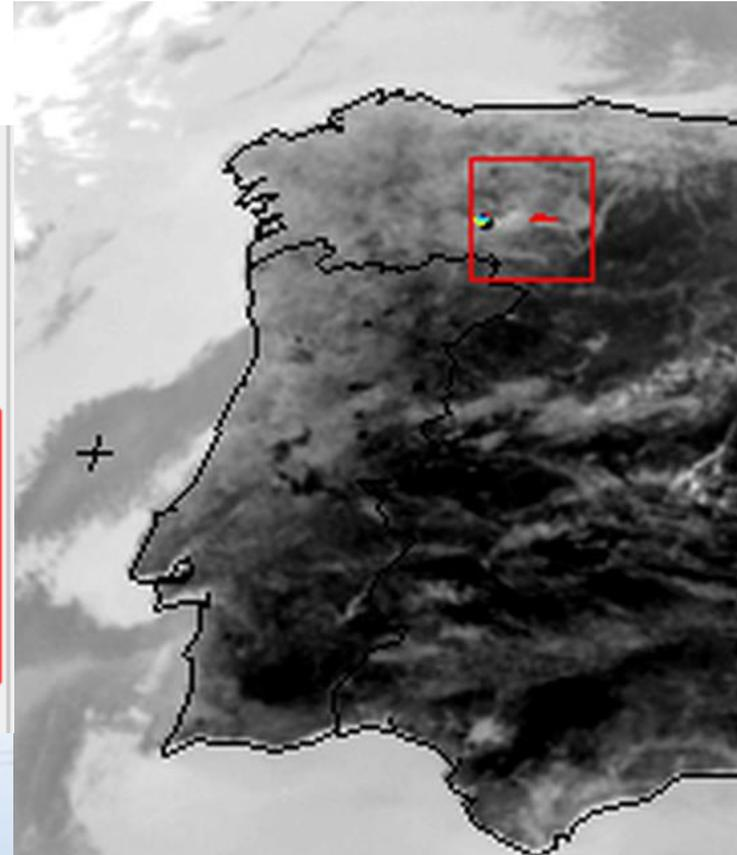
Fire fronts can increase the pixel albedo, first by the flames emission, later by changing the ground into a burnt surface, more reflective than a forest.
