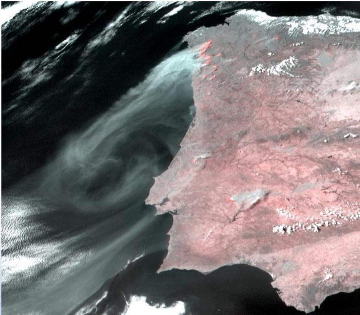
Meteosat: 30% of channel 3.9 $\mu$ m on top of HRV
