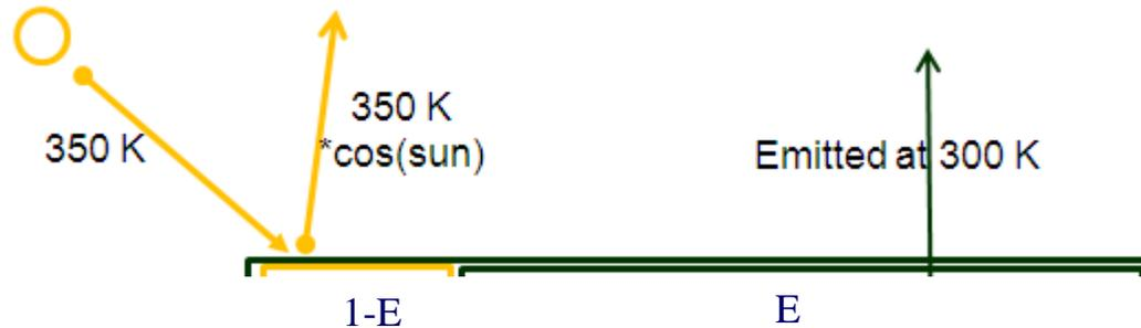
$$B(\text{BT}) = (1-E) * B(350\text{K}) + E * B(300\text{K})$$
