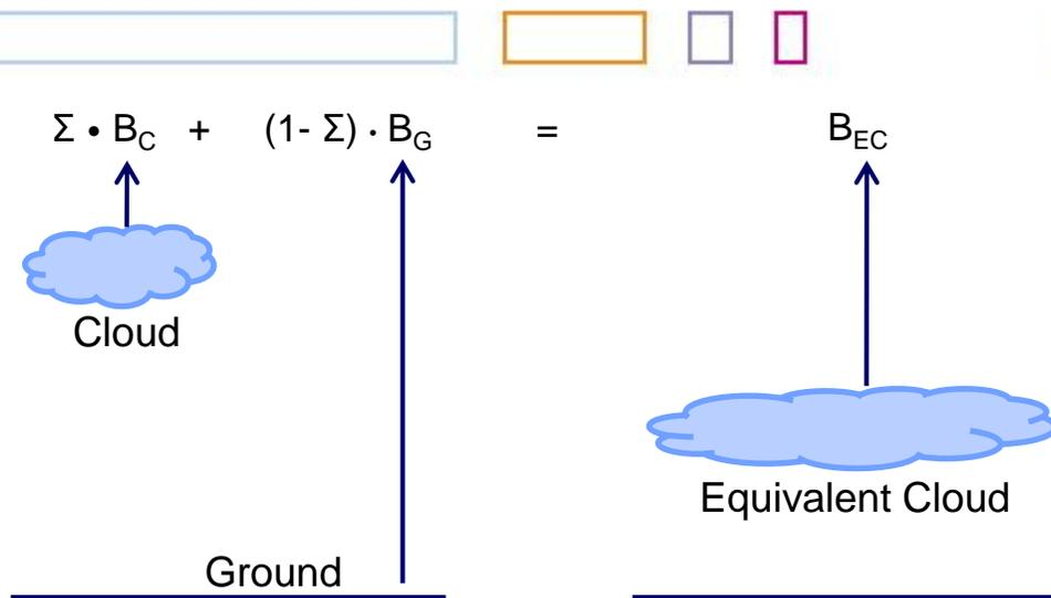
The equivalent temperature is not the average temperature, but shows a WARM BIAS!
