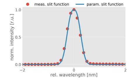
Slit function looks tame on the linear scale, but reveals all kind of structures on the log scale  $\rightarrow$  spectral stray light
