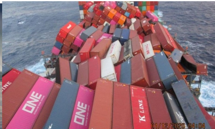
Container ship damaged by a storm in Pacific (Dec. 2020)
