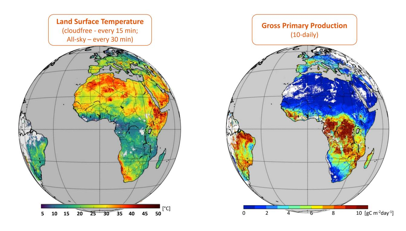
AVHRR/Metop provides Global coverage at c.a. 1km resolution: LST, Albedo and Vegetation State products. Set of variables will be extended with EPS-SG.
