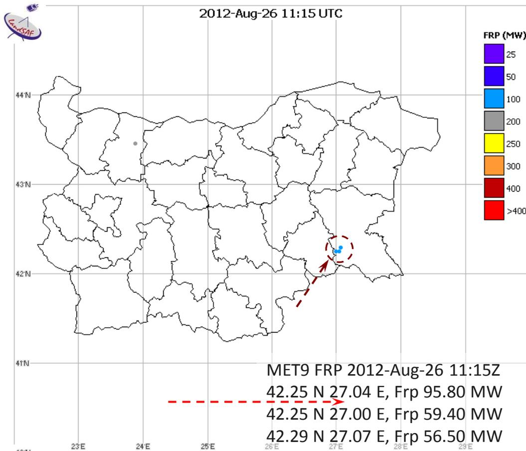
**At 1115 UTC MPEF FIR Full Scan did not detect the fire of pixels emitted FRP < 100 MW as derived by LSA SAF FRP product.**
