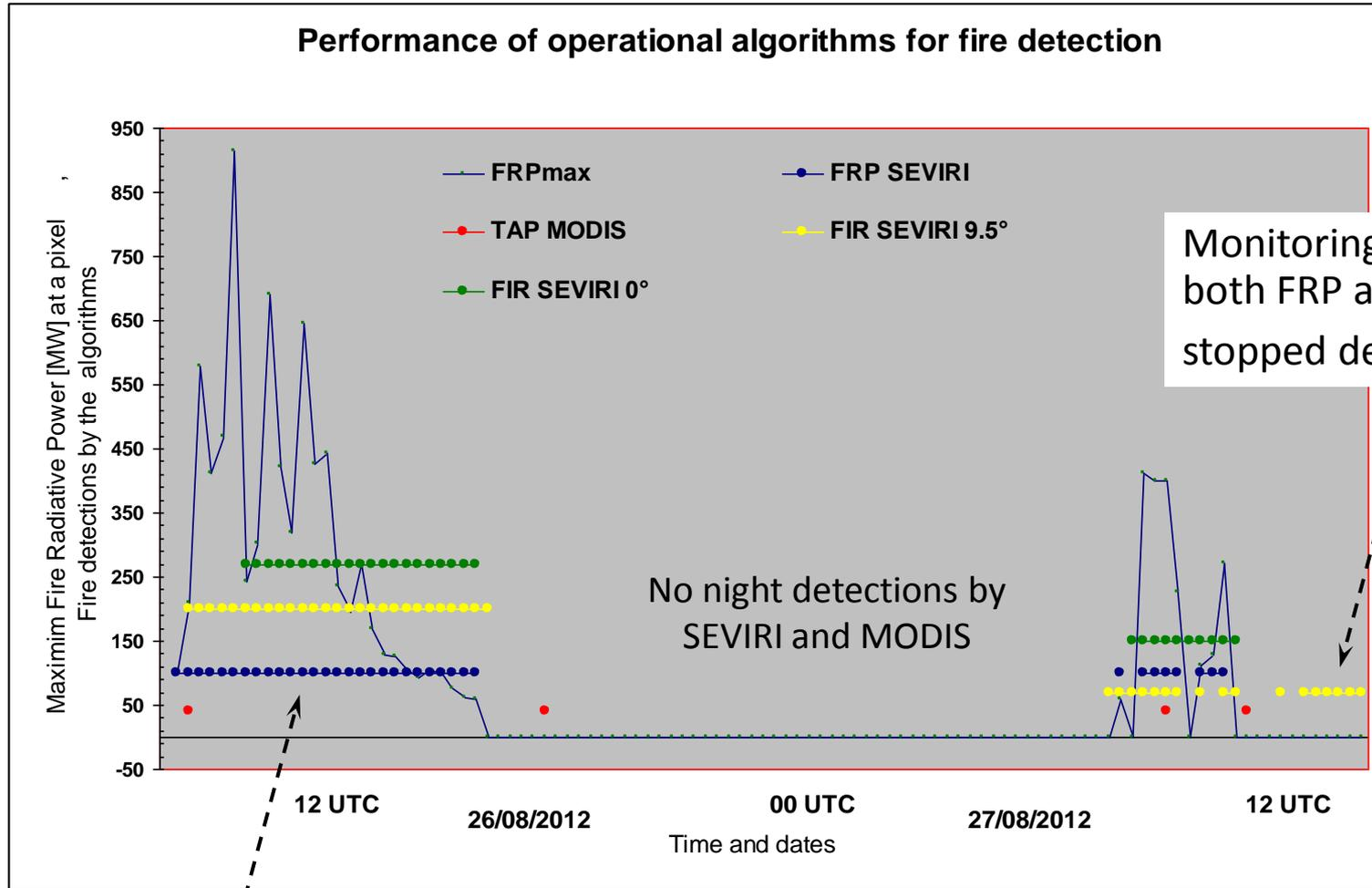
Fire detection by all products at the beginning of fire development and high Fire Radiative Energie (up to 900 MW) as measured by FRP product.
