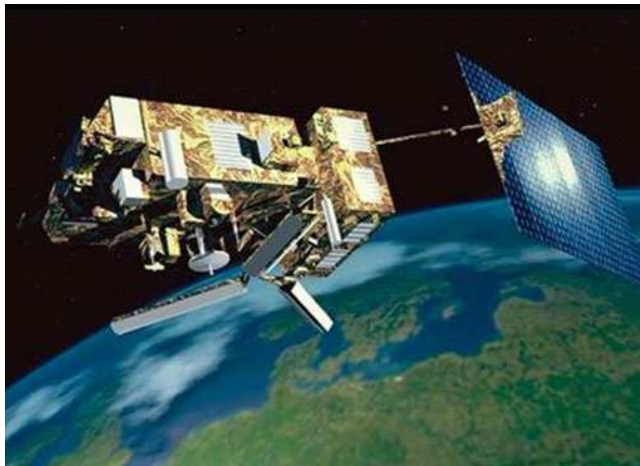
The Metop-A satellite carrying AVHRR imager with 6 spectral bands
